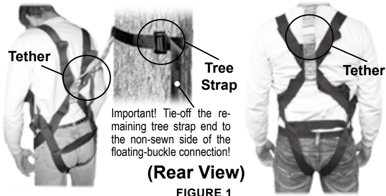
FIGURE 1 BIG DOG HUNTING FULL-BODY FALL ARREST SYSTEM (FRONT & REAR VIEWS)
